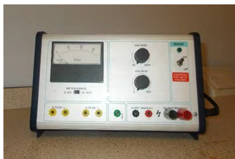
Figure 88: HT supply retrofitted with shrouded sockets
