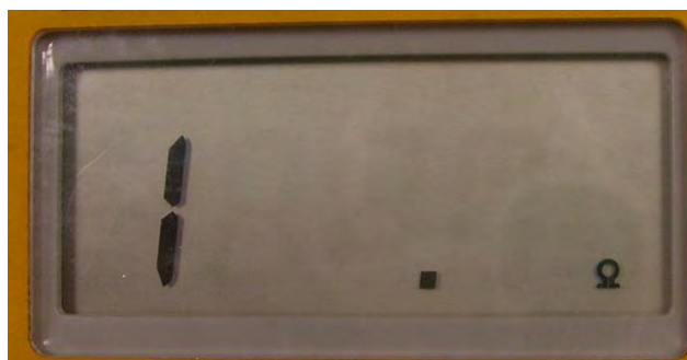
Figure 41: Meter displaying an 'Open Circuit' fault
