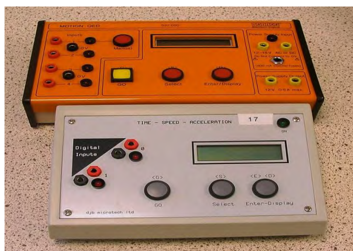
Figure 7: Timers with built-in microprocessors
