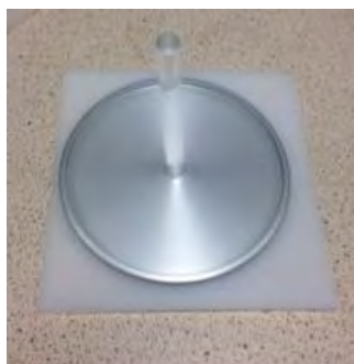
Figure 76: place the electrophorus on the slab
