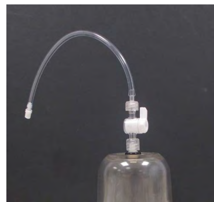
Figure 139: air tap on Student Bell Jar
