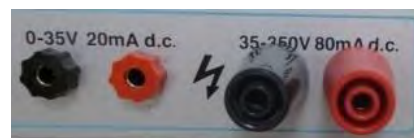
Figure 91: unshrouded and shrouded sockets
