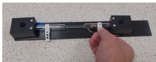
Figure 110: securing the tube with straps
