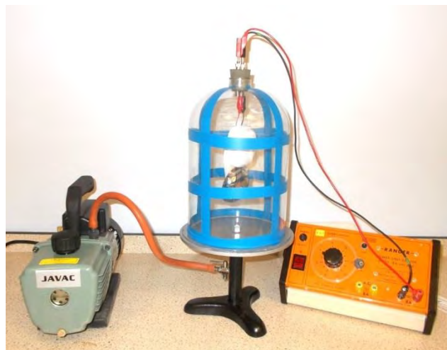
Figure 140: full-sized bell jar apparatus, set up to show the "sound in a vacuum" experiment.
