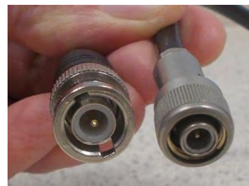
Figure 67: BNC (left) and PET 100 connectors
