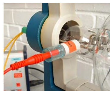
Figure 105: this collar is now fitted to the D-Series and can be retrofitted at school.
