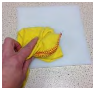
Figure 75: charge a polythene slab
