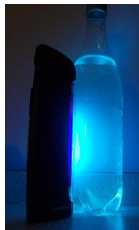
Figure 71: fluorescence in tonic water
