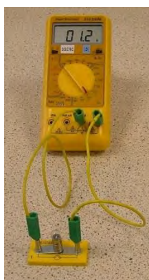
Figure 42: Testing a bulb using a meter
