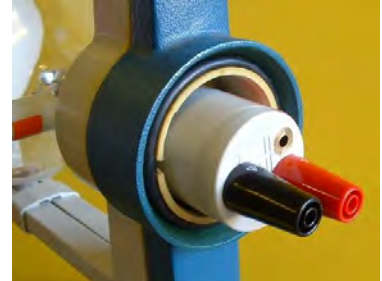
Figure 106: retro-fitted shrouded connectors to cathode / heater.
