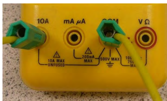
Figure 33: One lead in the COM (common) socket with the other in the 10 A socket
