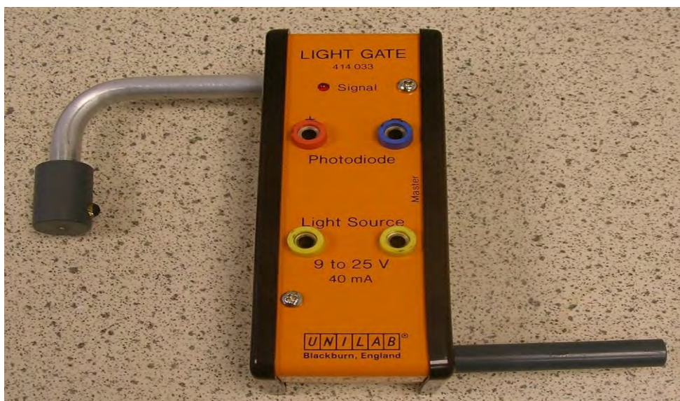
Figure 4: Combined light source and detector. The photodiode is the light detector.
